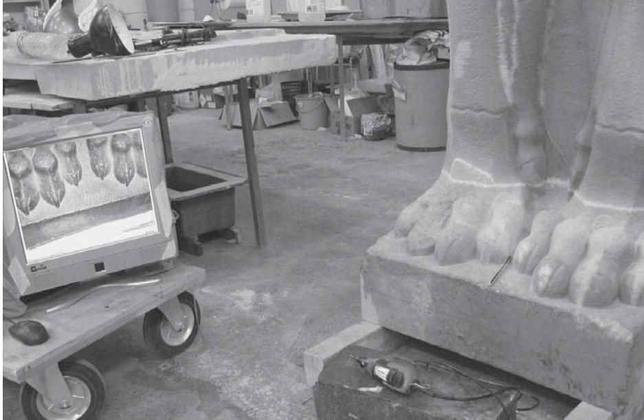
1.2 The feet of one of the human-headed lions from the entrance to the throneroom of Ashurnasirpal II now in the British Museum. The 3-dimensional data was recorded using a NUB 3D Triple White light scanning system and milled at a resolution of 400 microns. On the computer screen is an image of the scanned data which is directly compared to the facsimile to ensure accuracy. Photograph by Factum Arte
